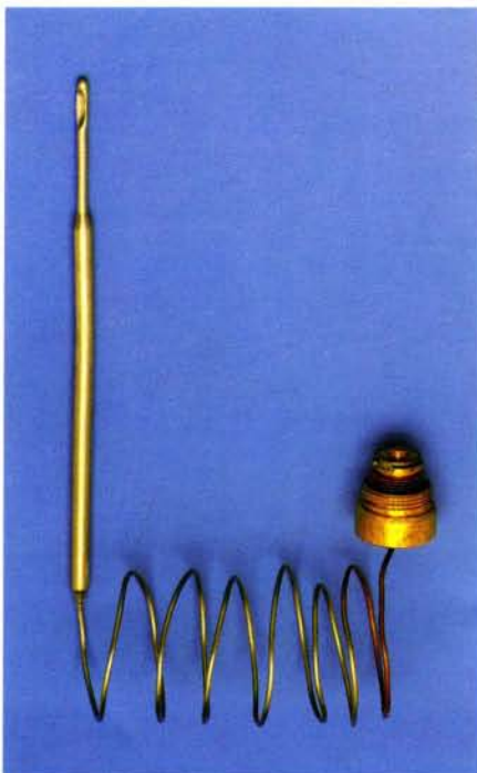
Due to the numerous deposit features there are more and more applications. Illustration shows temperature probe used in food industry
